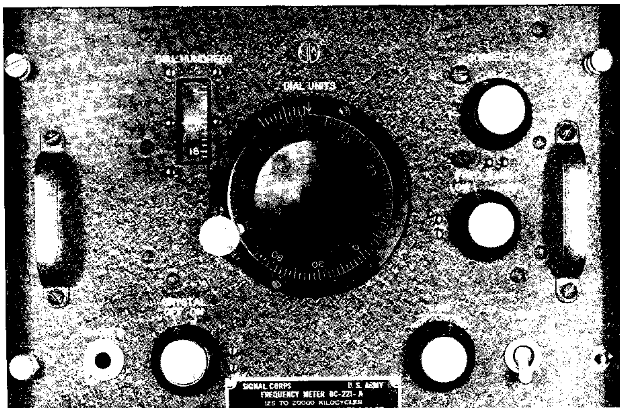
Figure 3. Frequency Meters BC-221-A, BC-221-C, and BC-221-D, control panel lay-out.
